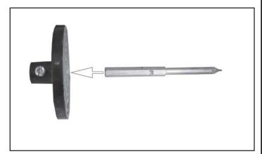
2. Hook the required hole saw onto the mandrel.
